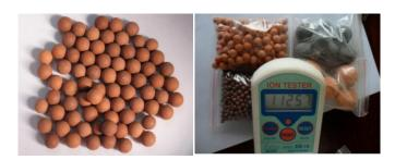
Negative ion ceramic ball is mainly made of the natural nonmetal mineral tourmaline, far infrared powder, kaolin and high-grade clay by nanometer comminution technology, special formula and agglomeration techniques. It emits far-infrared ray and negative ion which are good to the human body, Amount of generating negative ions: 1500~2000p/s.cm3, 3000~5000p/s.cm3,more than5000p/s.cm3.
