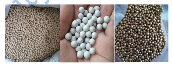
Antibacterial ball is made of nano silver antibacterial agent, tourmaline, Maifan stone, kaolin, clay etc. mineral materials by high temperature sintering.
