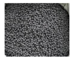
Magnetic energy ceramic ball is made of natural magnetic mineral materials(such as tourmaline, maifan stone, muyu stone, energy mineral powder) and other functional materials through high temperature sintering, which uniforms with a permanent magnetic particulate materials. It has a moderate magnetic field strength, broader magnetic field, high eradicate arc of magnetic line of force, etc.
