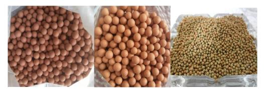
Far infrared ceramic ball is the special ceramic materials that can radiate specific wave infrared ray. It is made of variety natural mineral such as tourmaline, far infrared powder, kaolin etc. It is sintered by 1200 Degree C and become the Far infrared energy ceramic ball.
